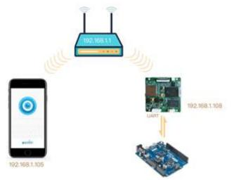
3) Module work as client and connect the router .APPs connect internet with 4G or a different router. the network have completed between module and APPs via internet. That will use Nabto P2P cloud server to interact data .
